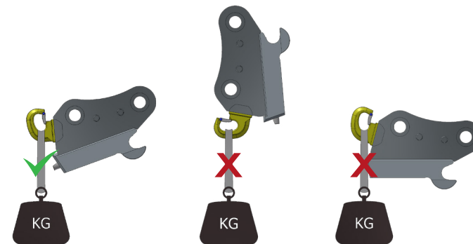
Fig. 16: Using the load hook
