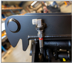
Fig. 10: Hydraulic line connections (example)
